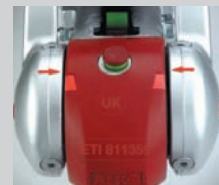
Friction Pads are worn out & need replacing
